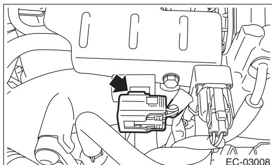
4) Remove the PCV hose assembly B from the intake duct.
